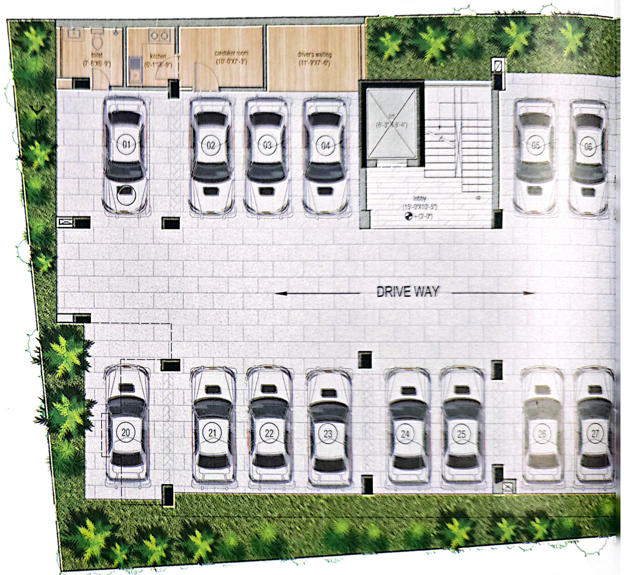
Ground Floor Plan (8536 sft) 11'-6" floor height ( 30 nos car )
